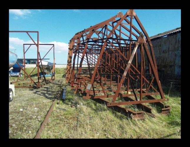
**Hull Forming Jigs at Offshore Steel Boats Ltd.**
